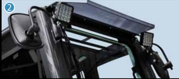
LED front lights (optional), rain visor (optional), and rear view mirrors (left & right)
