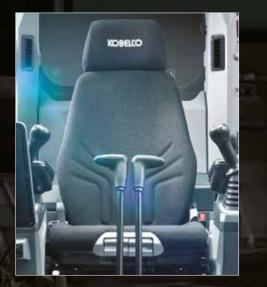
An air suspension sheet manufactured by the German GRAMMER AG comes as standard equipment. It has superior shock absorption and can be used for long periods of time without causing fatigue. The included armrest is 4 inches wide
