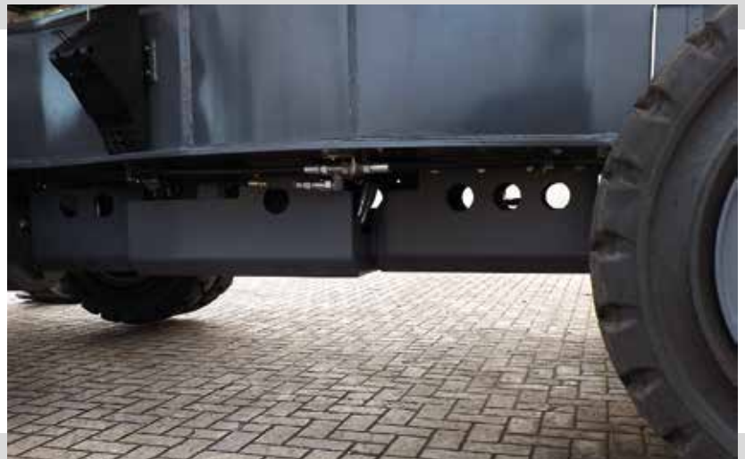
STEEL PLATES FOR THE UPPERCARRIAGE COVER BELOW
