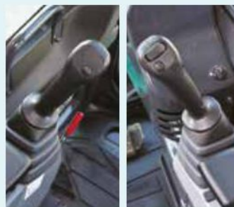
Proportional hand control lever for N&B piping (option) Precise proportional controls are integrated into the joystick for ease of operation.
