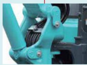
Hydraulic hosing The hydraulic hosing is housed inside the swing bracket.
