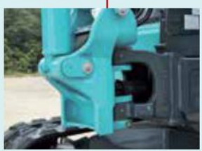
Swing bracket Large, thick cast-iron swing bracket/front bracket.
