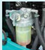
Pre fuel filter with built-in water separator
