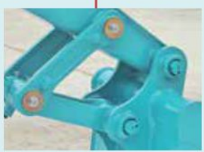
Bucket Cast-iron idler link provide greater strength.
