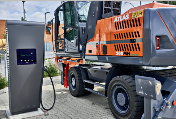
// Quickly recharged Direct current DC charging quick charging station CCS High charging power: 30 kW - 75 kW Charging time: 60 min. to 86% (SoC).
