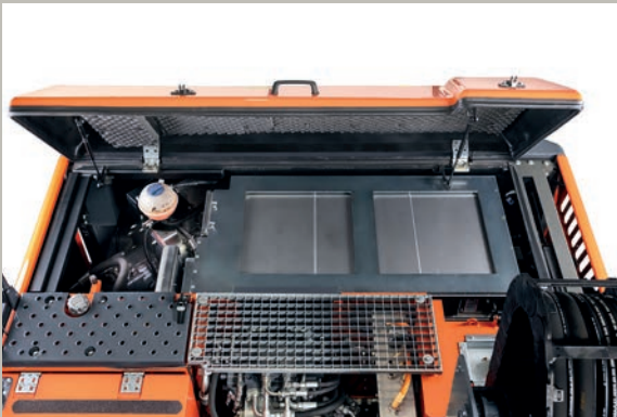
// Full power With our powerful battery at the rear of the machine, you enjoy an impressive operating time of up to 4 hours without the need to recharge. This innovative technology allows you to work longer and more efficiently, without interruption for battery change or recharging.
