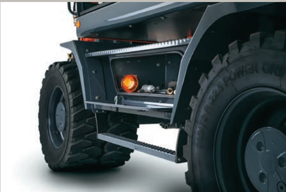
// Tools always on board In the toolbox on the undercarriage all kinds of tools are stowed ergonomically arranged for quick use on site.
