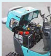
Fully opening hood for large access space.
