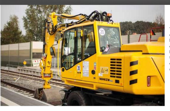
The low centre of gravity and our compact design guarantee high stability with excellent off-road mobility. 1604ZW also has a bilateral barrier on the track wheel cylinder at a swing of 5° from the longitudinal axis and at a standstill.
